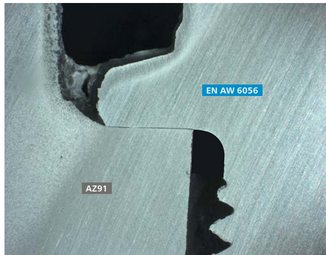
Contact area of Alufast® screw (EN AW 6056) and housing flange (AZ91) after 720 hours salt spray test (ISO 9227)
