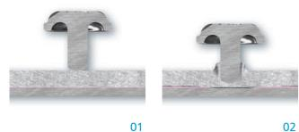
Press the components together, provide the fastening element 02 | Penetration
