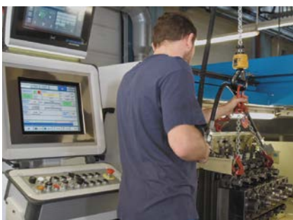
A worker installs the tool block, which has been prepared in advance outside the machine.
