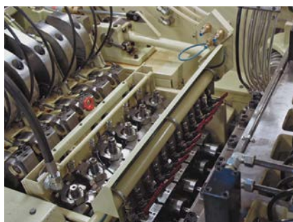
The parts are gradually brought into the desired shape via various forming stages.
